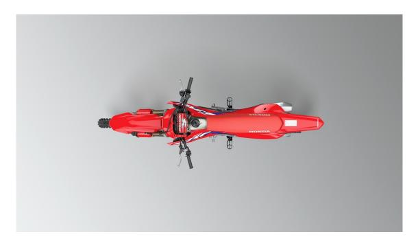
Model updates: Mechanically unchanged for 23YM the CRF250R is still the strongest it's ever been; in 22YM it got the MXGP championship-winning chassis of the CRF450R plus extensive cylinder head development for a considerable low-rpm torque boost. Cooling efficiency was also improved, while a strengthened gearbox got revised ratios and nine-plate clutch. A new graphic treatment marks out the 23YM machine and features a brand new redesign of the iconic HRC logos.
